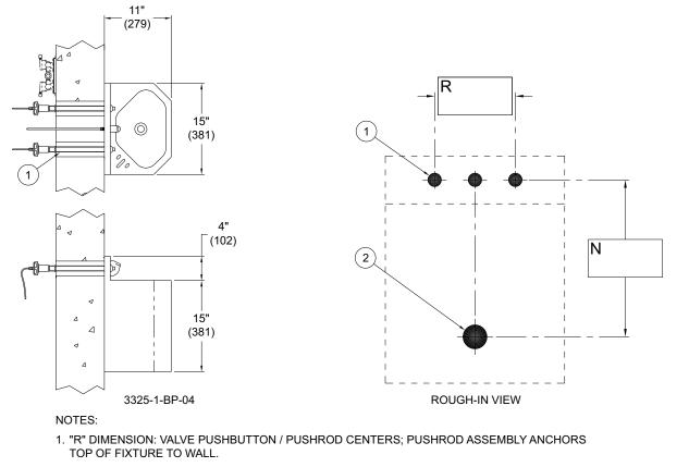
2. "N" DIMENSION: LAVY WASTE OUTLET LOCATION. 9" MINIMUM FOR ELBOW WASTE OUTLET AND 8" MINIMUM FOR OPTIONAL -PT P-TRAP OUTLET. MUST SPECIFY.
