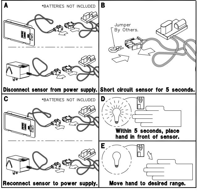
NOTE: THESE INSTRUCTIONS ONLY APPLY TO 9 VOLT SENSORS THAT DO NOT HAVE A RANGE ADJUSTMENT SCREW ON THE BACK. SEE DRAWING # 9927-222-001.
