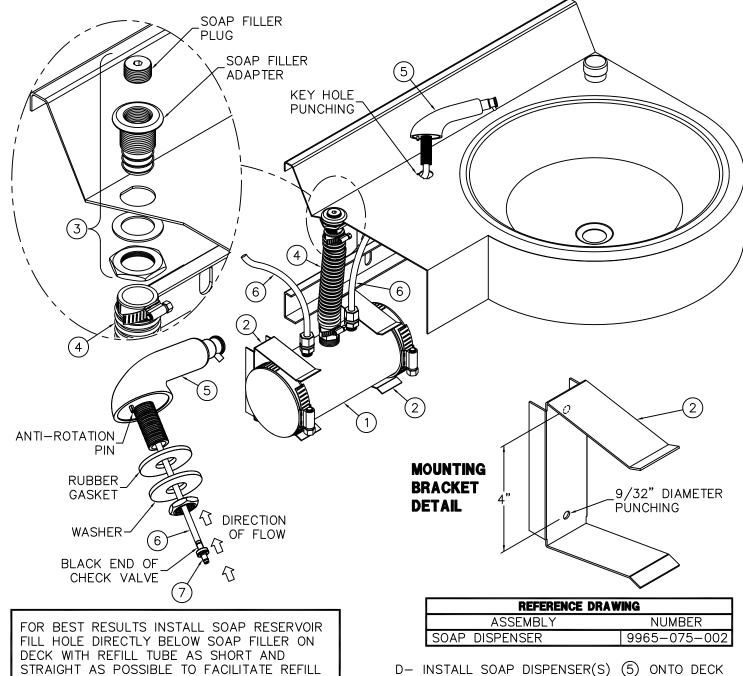
A- INSTALL SOAP RESERVOIR (1) TO WALL INSIDE THE TRAP ENCLOSURE USING THE MOUNTING BRACKETS (2) PROVIDED. WALL ANCHORS AND FASTENERS ARE BY OTHERS.
