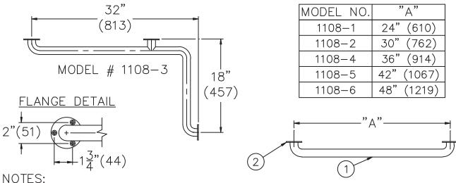
1. 1-1/2" O.D. Stainless Steel Tube. 2. 3" O.D. Stainless Steel Flange.
