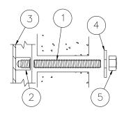
MOUNTING DETAIL FOR 1/4' STUDS
