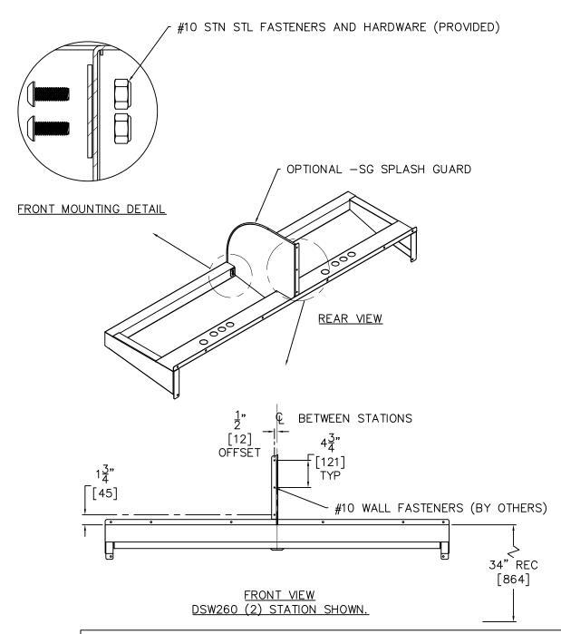
NOTES: OPTIONAL -SG SPLASH GUARD IS LOCATED ON CENTERLINE BETWEEN STATIONS. REFER TO APPLICABLE SUBMITTAL FOR DIMENSIONAL DATA AS REQUIRED FOR 2, 3 AND 4 PERSON UNITS.
